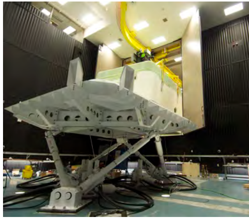
Moving the General Purpose Payload onto the Motion Base
